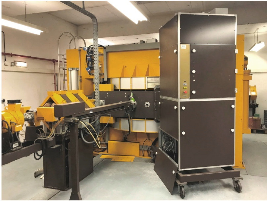
Figure 2: Scanditronix MC-60PF Cyclotron and first quadrupole triplet.
