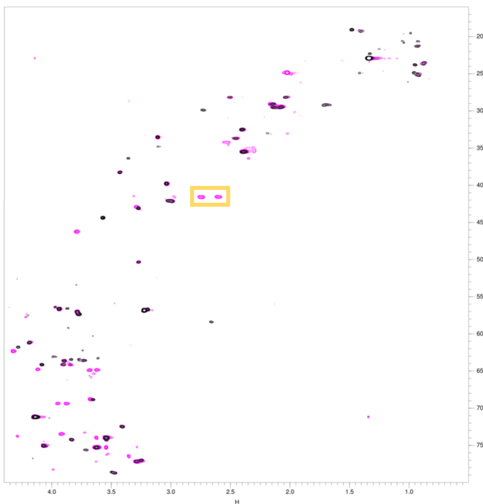
Fig 4.15 A 2D HSQC ^1\text{H} - ^{13}\text{C} spectrum of the aliphatic region of IDH WT (black) and IDH Mut (pink) overlaid. The yellow box indicates the location of the 2-HG peak. Here the ^1\text{H} resonance can be seen on the x-axis and the ^{13}\text{C} resonance on the y-axis.
