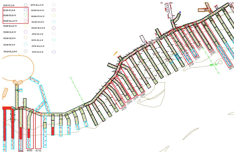
Figure 13: Support classes in the research area at Level 1051 and 1052 with marked crosscuts (MicroStation V8i)
