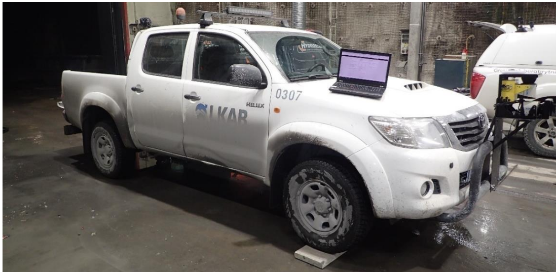
Figure 39: Calibration procedure with wood under the front wheels
