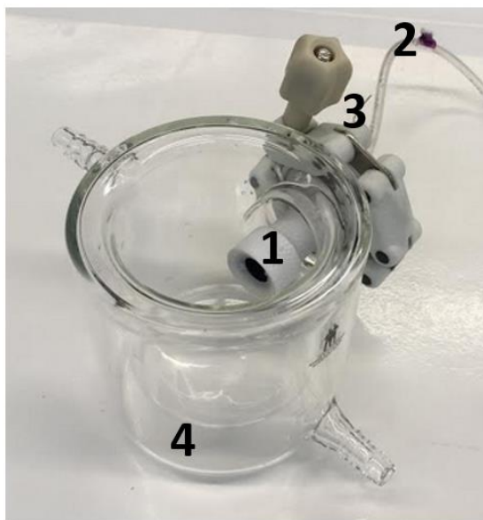
Figure 12 Gas diffusion electrode setup: 1) GDE; 2) gas tube; 3) current collector; 4) electrochemical cell.
