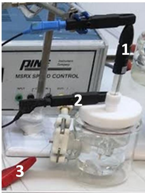
Figure 13 Gas diffusion electrode setup connected to the potentiostat: 1) counter electrode; 2) reference electrode; 3) working electrode.
