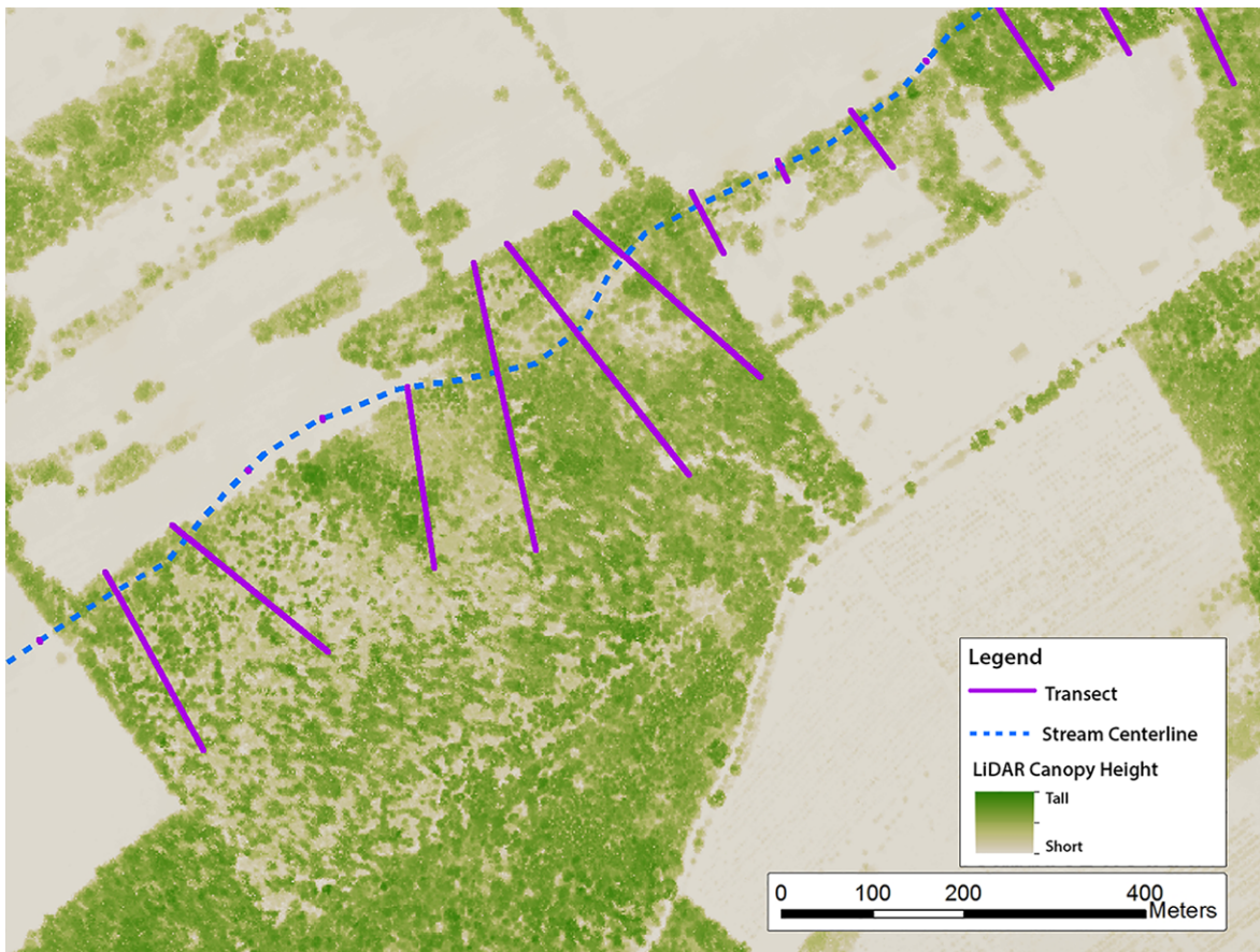
Fig. 2. An example stream segment and associated transects. The algorithm processed each transect on either side of the stream separately. Each transect was then used to estimate buffer width and quantify vegetation structure throughout the Spring Creek watershed.
