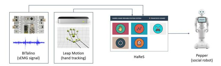
**Figure 1.** Architecture of HaReS, a hand rehabilitation system, featuring surface electromyography (sEMG) and hand tracking low-cost sensors.
