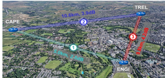
Figure 2. The Cambridge quantum network, connecting the University of Cambridge’s Electrical Engineering building (CAPE), Engineering dept (ENGI) and Toshiba Research Europe (TREL). Fibre lengths range from 5.0 to 10.6km, with losses between 2.5 and 4.2dB. Credit Dynes et al 32 .
