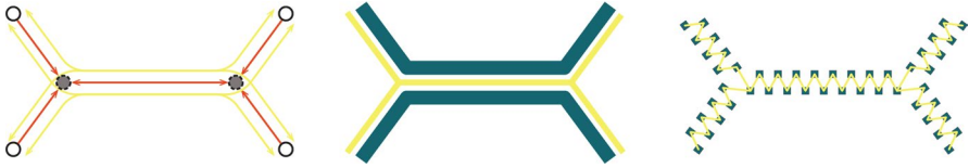
Fig. 7 The dwelling block and its formal resemblance to a Euclidean Steiner diagram. Intermediate nodes aim at minimizing the paths between endpoints but at the same time they maximize social interaction. The internal logic of the apartment arrangement can be a subsystem of crinkled circulation
