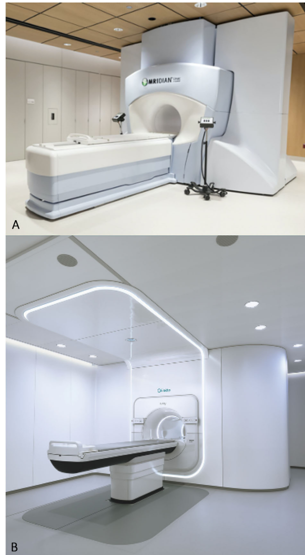
FIGURE 2 | The two commercially available MR-guided radiotherapy systems. (A) The MRIdian (ViewRay Inc, USA). (B) The Unity (Elekta, Sweden).
