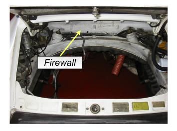
Figure 5.3: Location of firewall within the engine compartment.
