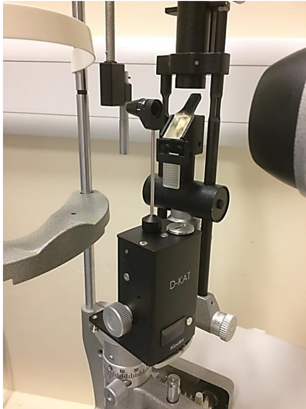
Fig.16. The T type D-KAT Goldmann applanation tonometer (Keeler UK) used by the present study, mounted on a slit lamp.
