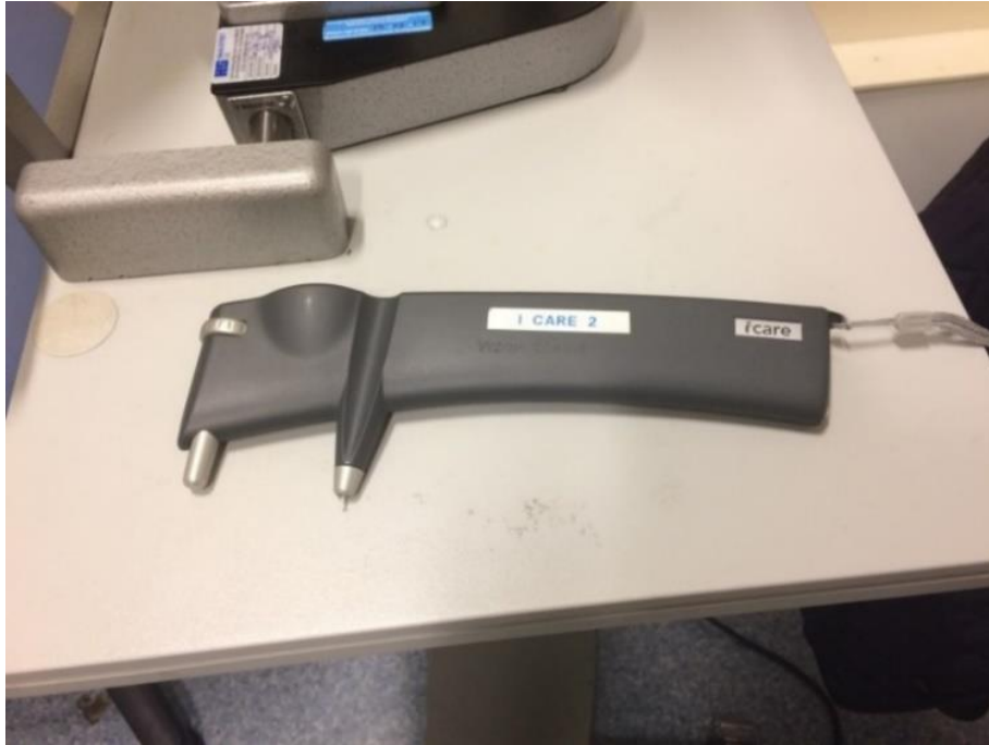
Fig. 20. TA01i Icare tonometer used by the present study. The photograph shows the probe in situ.
