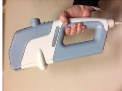
Fig.14. The Keeler Pulsair IntelliPuff tonometer (PT00) (Keeler Ltd, Windsor,UK) can be used in the supine position. It is small, portable and easy to use. Therefore, it can be used by non- ophthalmic colleagues (Vernon et al. 1990).
