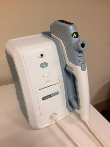
Fig.14. The Keeler Pulsair IntelliPuff tonometer (PT00) (Keeler Ltd, Windsor,UK) can be used in the supine position. It is small, portable and easy to use. Therefore, it can be used by non- ophthalmic colleagues (Vernon et al. 1990).
