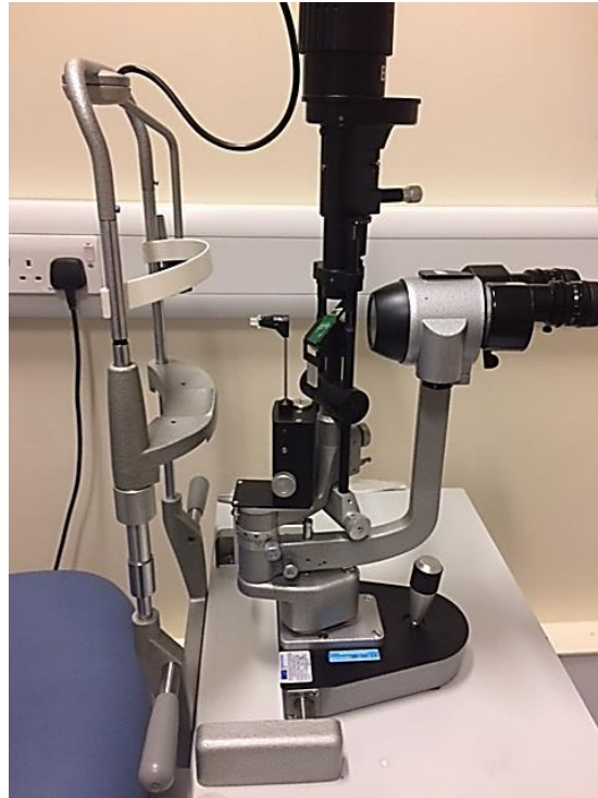
Fig. 28. The Haag-Streit slit lamp (Haag-Streit UK Ltd) with T type D-KAT Goldmann applanation tonometer (Keeler UK) used by the present study.
