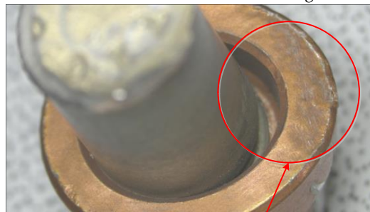
Obvious plastic deformation on the nut
