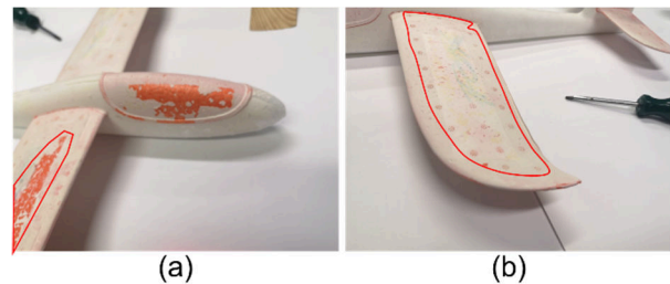
Figure 3. The details of the target aircraft model. The red areas are the damaged area. (a) refers to the right-wing and node, (b) refers to the left-wing.
