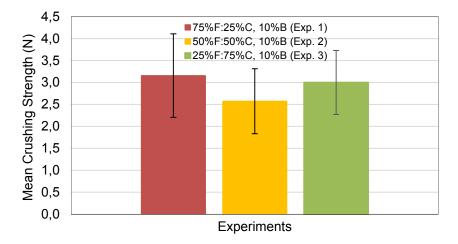
Figure 2: Mean crushing strength of 500 - 600 µm granules at different powder ratio with constant 10 % of binder
