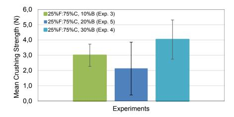
Figure 6: Mean crushing strength of 500 – 600  $\mu$ m granules at different binder percentage and constant powder ratio of 1/3 (25 % Fine: 75 % Coarse)
