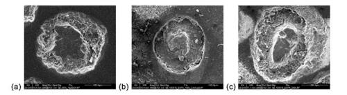
Figure 8: SEM images 200× of granules at constant powder ratio of 1/3 (25 % Fine: 75 % Coarse); (a) 10 % binder 200×, (b) 20 % binder 100×, and (c) 30 % binder 200×
