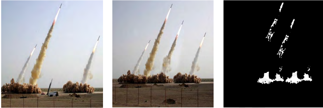
Figure 1.8: A typical copy move forgery, applied to a press photograph of an Iranian missile test. The original image with three missiles (shown on the left). The forged image with four missile using copy move attack (shown on the middle). The right image shows the detection results.
