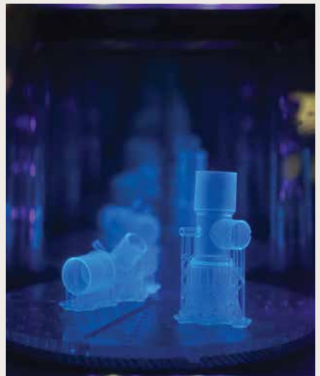
3D-printed ‘exhalation ports’ used in the patient circuit of a ventilator system.
