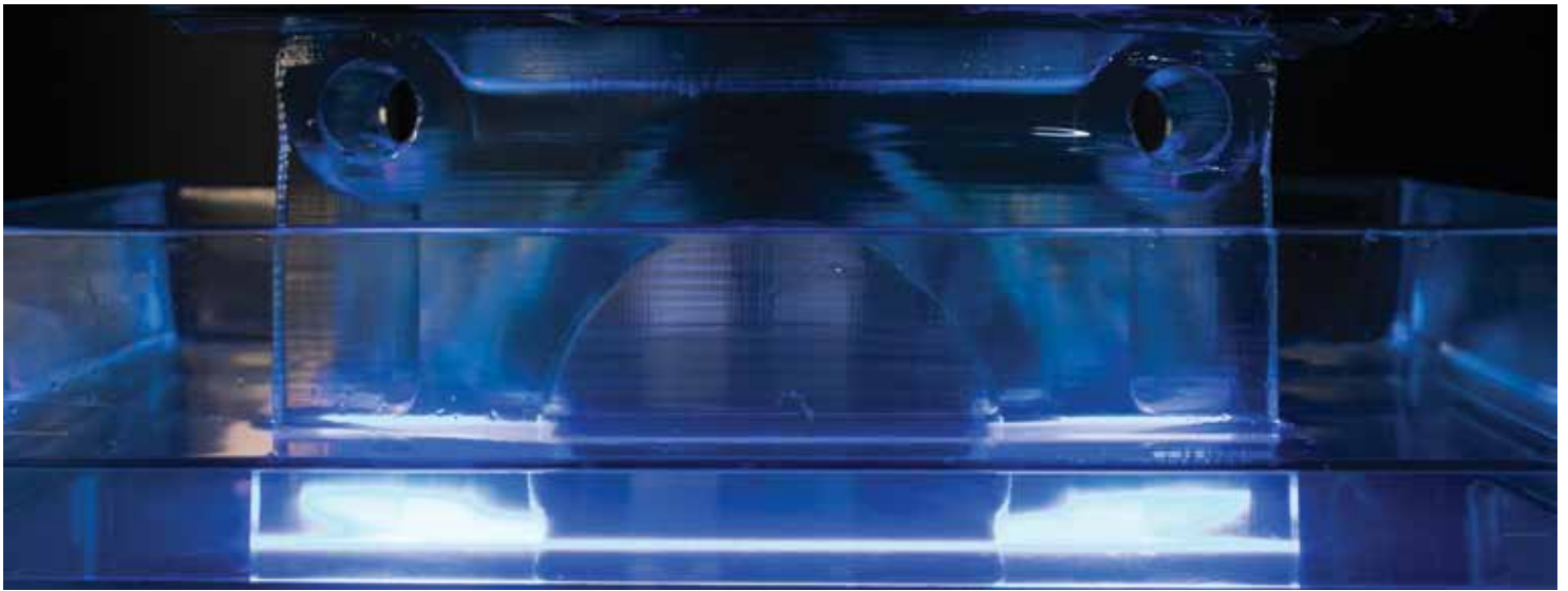
A prototype face mask mold, designed by collaborators at Brown University, is shown inside one of Phillips' 3D printers. The solid material of the part is cured by layers of ultraviolet light projected inside a bath of photopolymer resin.
