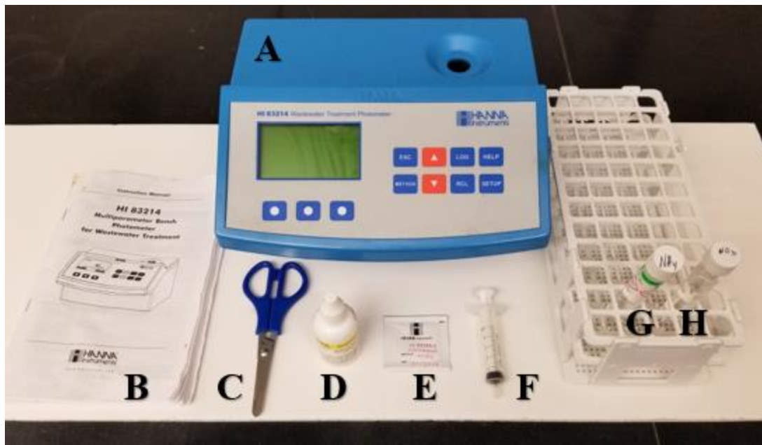
Fig. 2 Multiparameter bench photometer and supplies: photometer (A), instruction manual (B), scissors (C), Nessler's reagent (D), powdered reagent (E), syringe (F), ammonium test vial (G), and nitrate test vial (H)
