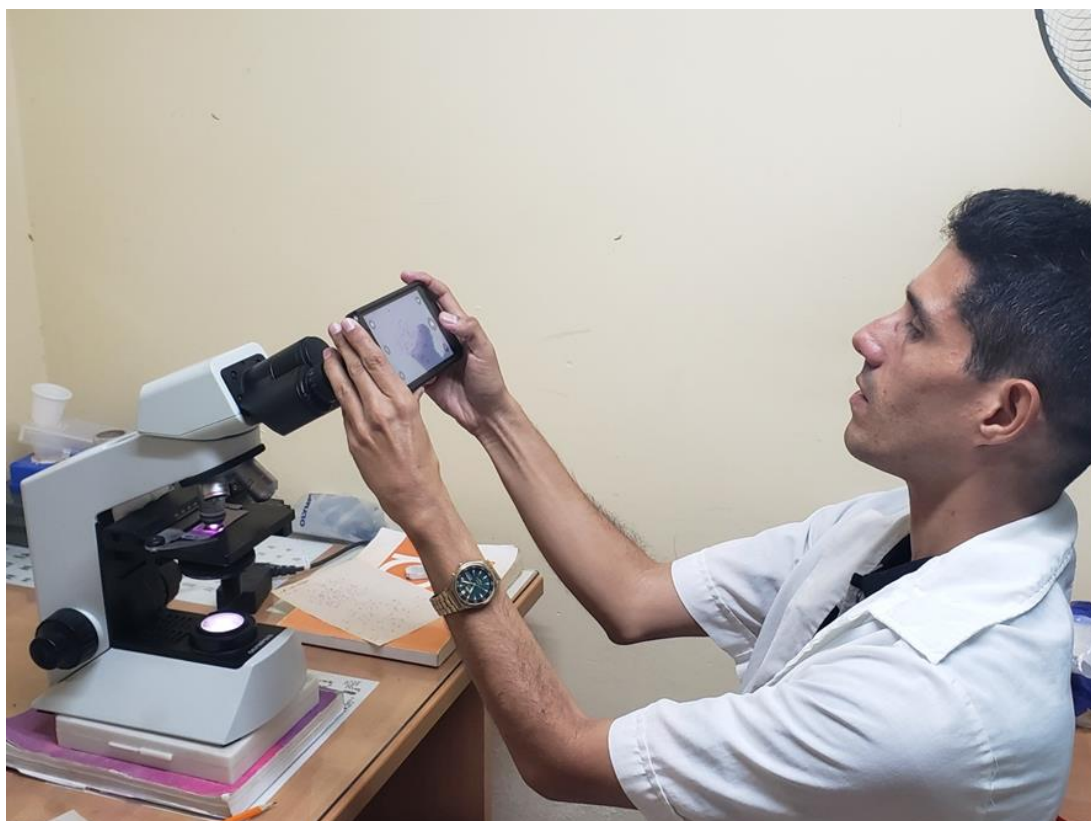
Fig. 3. Researcher capturing an image with a smartphone through the eyepiece of a microscope
