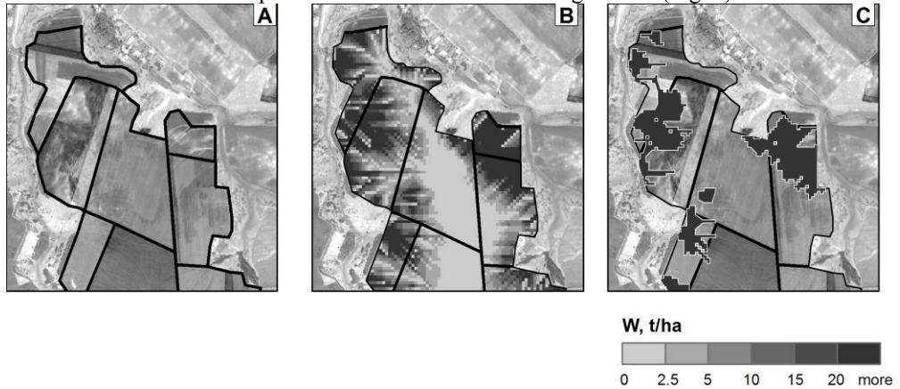
Fig. 1. Steps for identifying areas of high erosion hazard: A – view of arable land in a satellite image; B – simulation results of the soil losses caused by erosion with water fallow field; C – identification of areas of high erosion risk (more than 20 t/ha per year).
