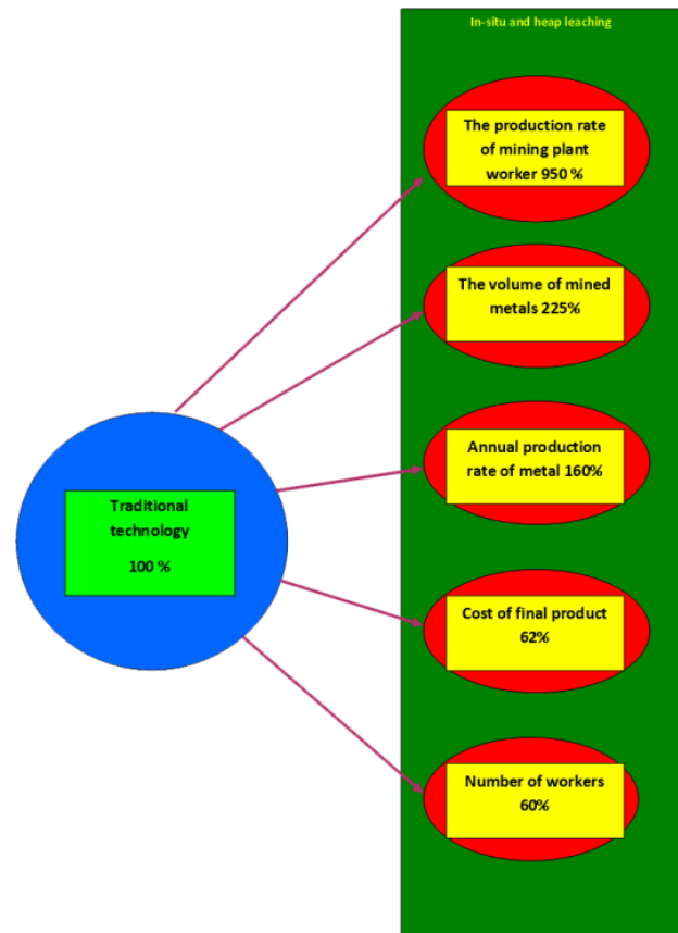
Figure 5. The effectiveness of in-situ leaching of ores
