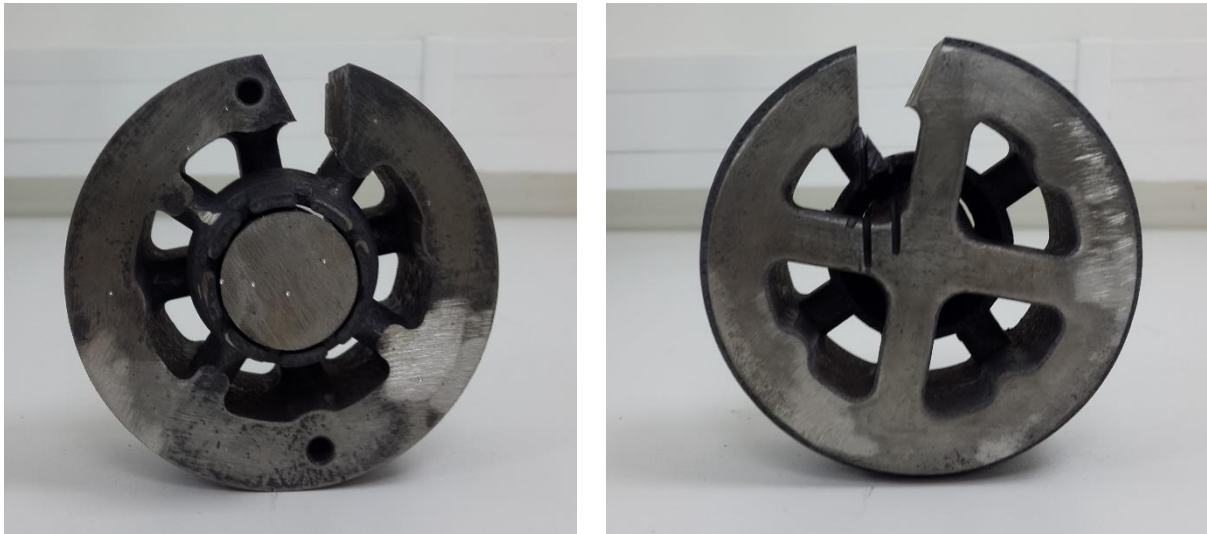
Figure 3. Solid die with simple geometry produced by DMLS.
