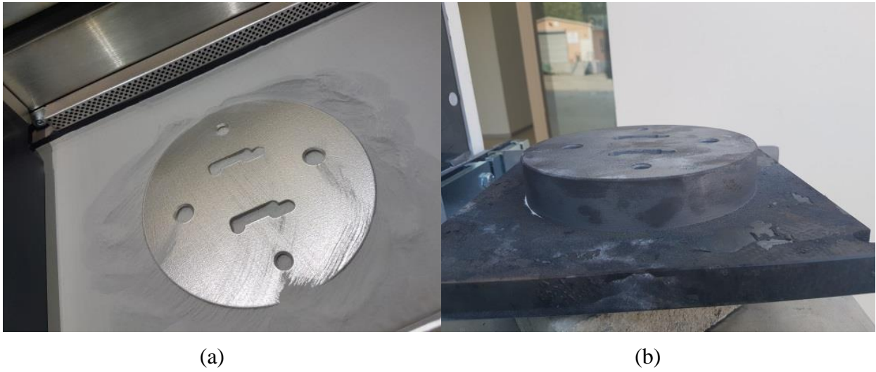
Figure 4. Extrusion die, (a) as produced in EOS M290 machine and (b) after stress relieving.
