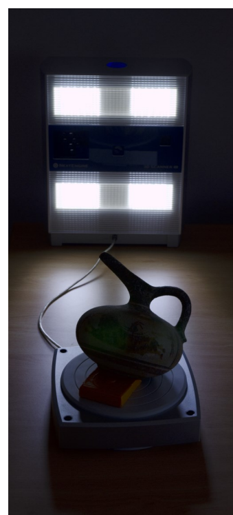
The colour is captured through LED lighting and an internal camera.
