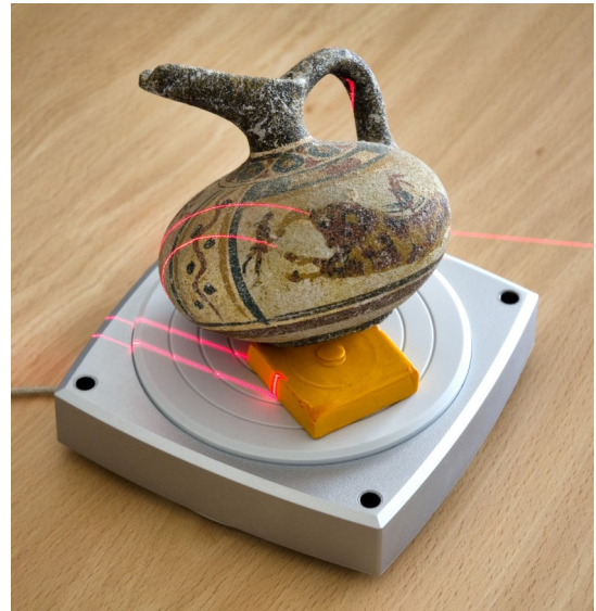
Scan in oblique position to cover areas not visible in other positions.
