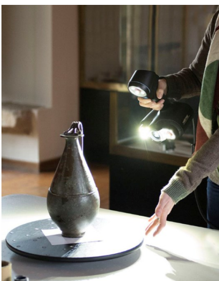
3D scan using the light scanner structure of the Jarro de Siruela (6th century BC), which is located in the Archaeological Museum of Badajoz.
