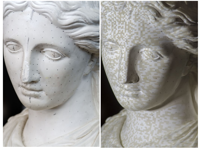
Projection of a structured light pattern on the surface of the object.
