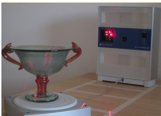
Scanning a Roman glass cup reproduction by using the NextEngine desktop scanner.
