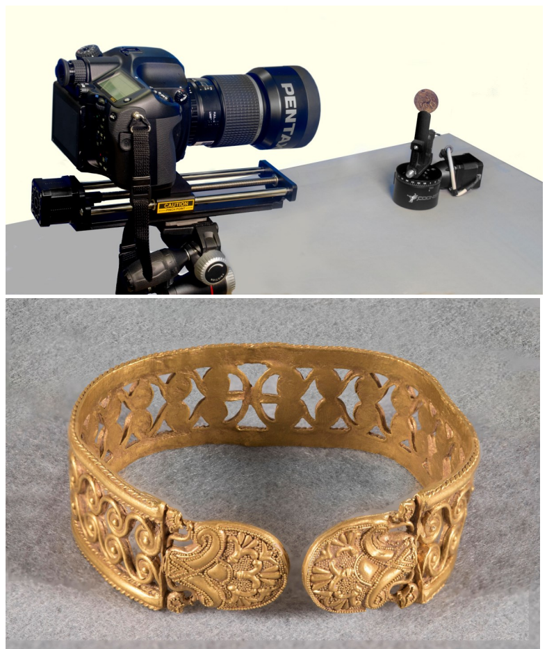
Example of an image generated using focus stacking can be seen here (Ref. MAN 2855).
