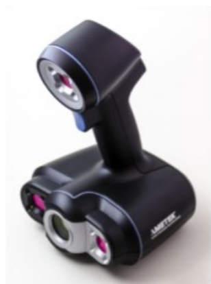
Photoshoot preparation (above), Pentax 645Z camera and Go!Scan structured light scanner (below).
