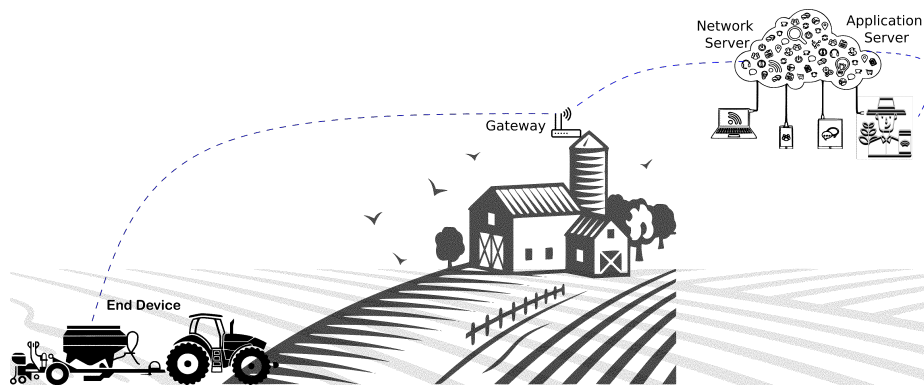
Fig. 1. A High-level view of agricultural telemetry system architecture based on LoRaWAN. The system is composed of five essential elements: End-Device , Gateway , Network Server , Application Server and Applications .
