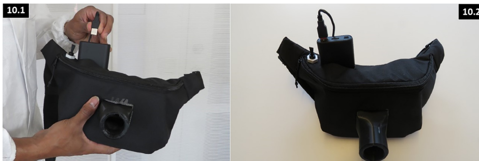
Fig. 15. (Left to right) Procedure to complete the power supply and conditioning unit.
