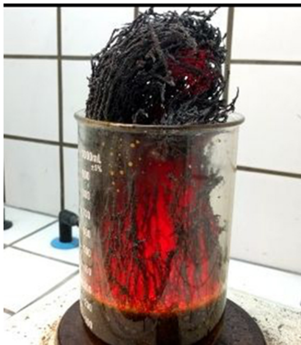
Fig. 2.3: Exothermic reaction during sol-gel autocombustion method.
