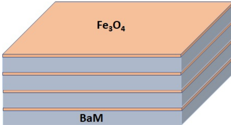
Fig. 6.7: Schematic of the model used for coated BaM with Fe 3 O 4 layers. Each layer of BaM nanoparticles is coated with 1, 2, or 3 layers of Fe 3 O 4 films or nanoparticles.
