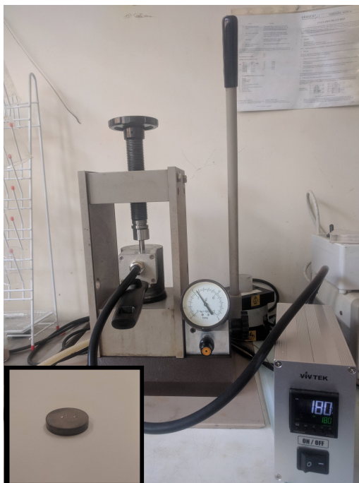
Fig. 2.5: Warm compaction setup and the form bonded magnet sample.
