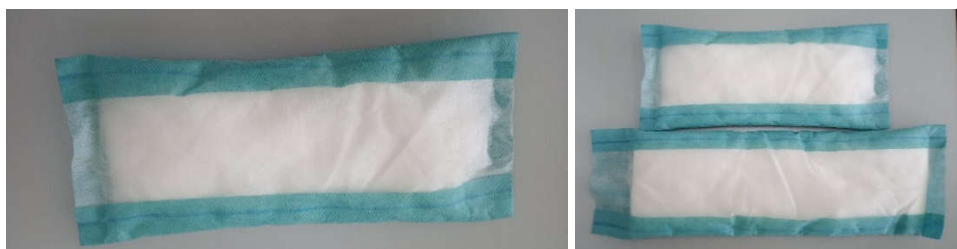
Figure 69 - Prototype of a medical obstetric pad made of E. globulus bleached kraft fluff pulp.
