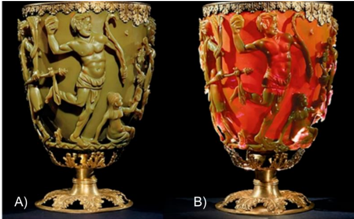
Figure 1.1 - The Lycurgus cup, stored in the British National Museum. The cup appears mate green in direct light (A) and red if light shines through it (B). Picture adapted from Bayda et al. (2020).
