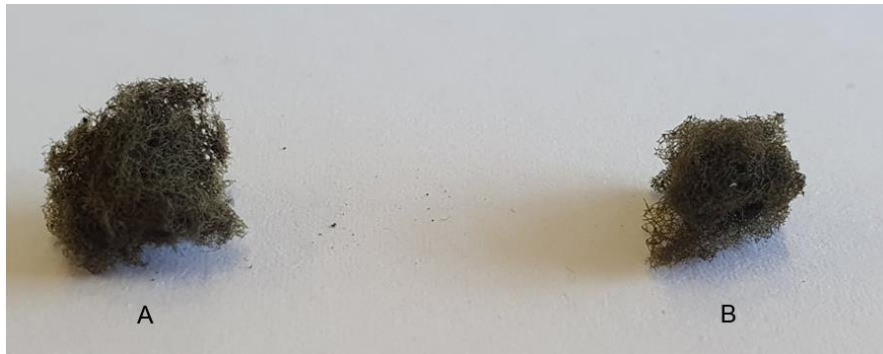
Figure 45. Image of the (A) 3xPEI/GO and (B) 3xPEI/rGO scaffolds with thermal treatment at 180° C under vacuum (12h).
