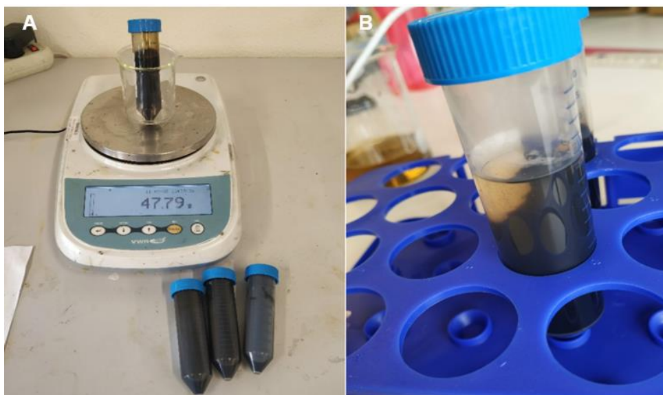
Figure 12. Purification of the GO using ultrapure water, before A) and after separation by centrifugation B).
