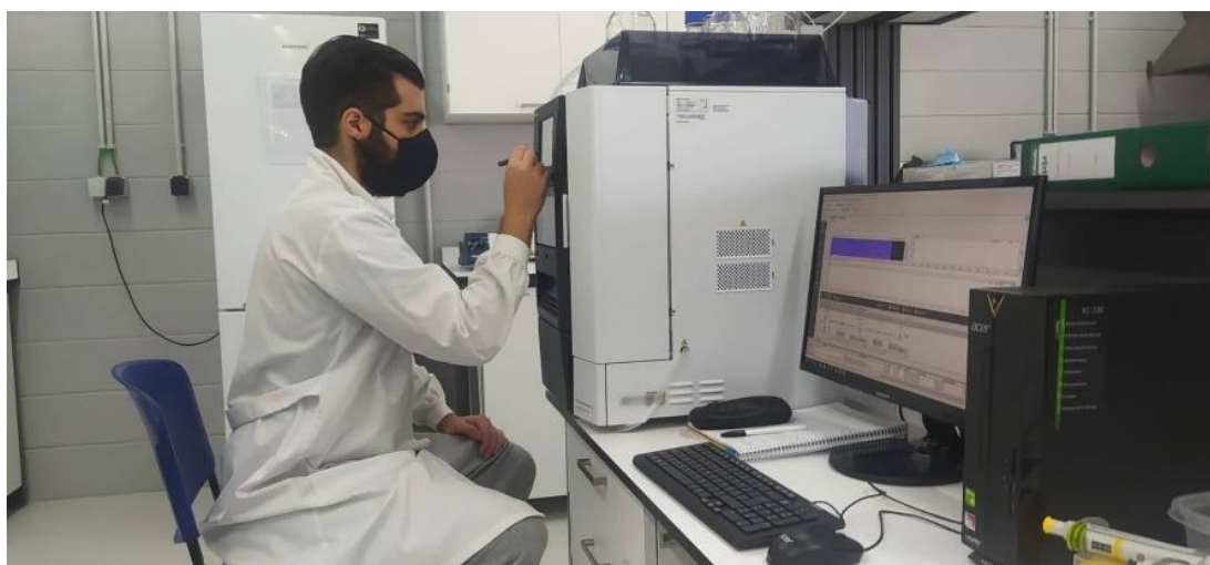
Figure 14 – Identification of photosynthetic pigments performed using a Shimadzu HPLC.
