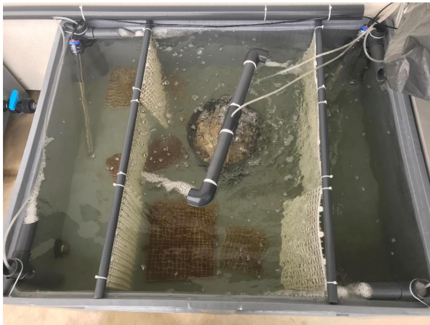
Figure 12 – Airlift system used to keep Exaiptasia diaphana on the dark to bleach them.
