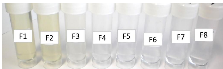
Figure 2.4. Detail of colour change of extracts along fractions collected during MHG experiment of iBB 6.
