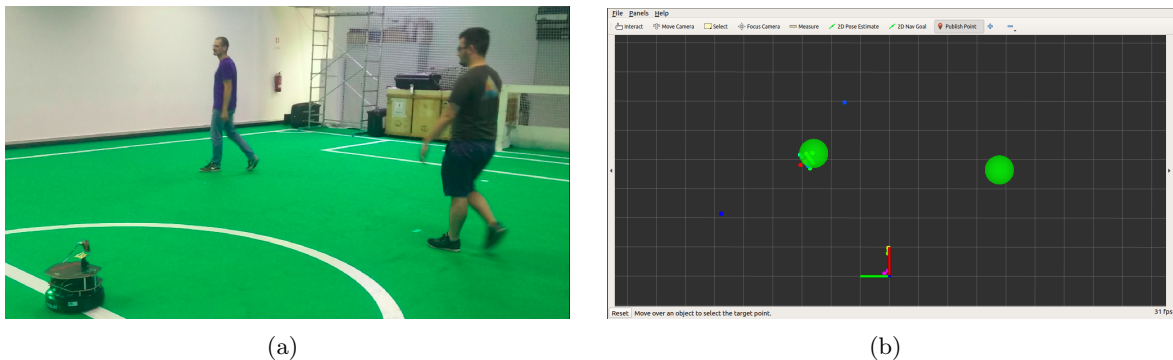
Figure 6.10: Two people walking in front of the static sensor (left) and the graphical representation of this experiment in rviz (right).
