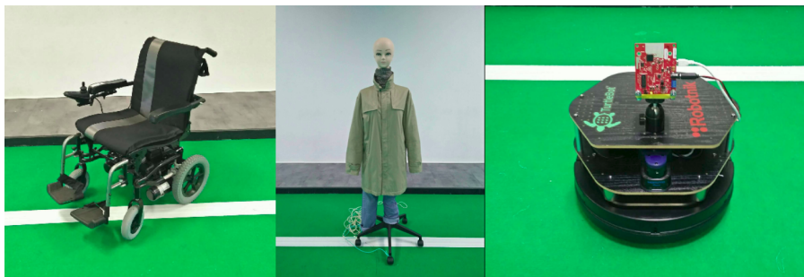
Fig. 2. Wheelchair (left) and mannequin (center) used in the tests. TurtleBot with radar installed on its top (right), with an upward inclination of 10 degrees.
