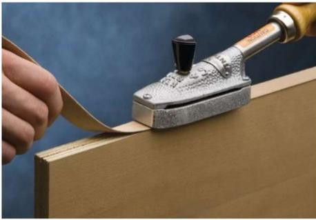
Figura 44: Processo de “edge banding”
