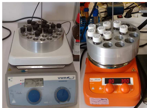
Figure 20. Solubility assay of LMMCs (left) and technical lignins (right).
