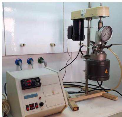
Figure 22. PARR Stirred reactor 4843 (300 ml of capacity).
