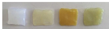
Fig. 1. Macroscopic appearance of the wet BC membranes incorporating the different ILs. From right to left: BC, BC-[Chol][Caf], BC-[Chol] 2 [Ell], BC-[Chol][Gal]. The produced membranes had a water content of 62.12 ± 4.40%.
