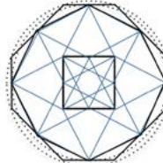
seed octagon and octagon of grid of two together with seed square in the middle
