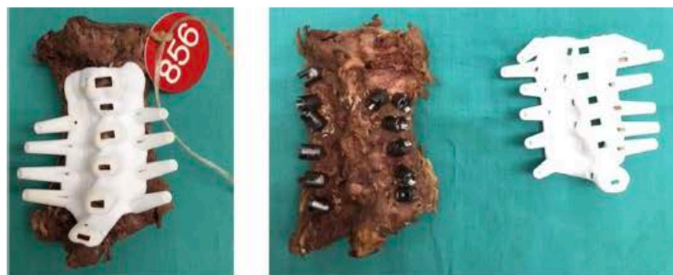
Figure 4. Intraoperative images of the templates. Left image; example of how the template adapt to the cadaveric cervical column.
