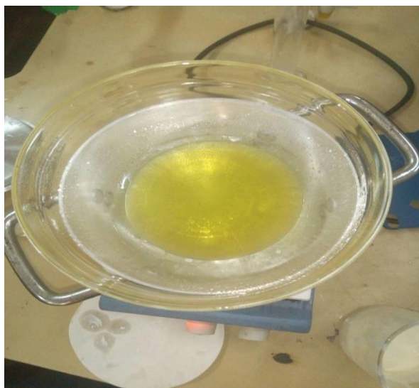
Figure 2.1 Blending of the base oils over a double boiler
