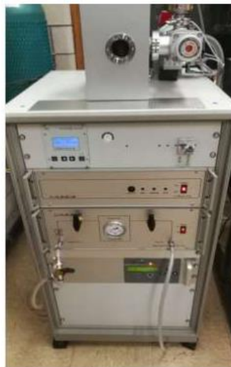
Figure 8 Equipment Used for Dilatometry Tests (LINESEIS L78 Machine)
