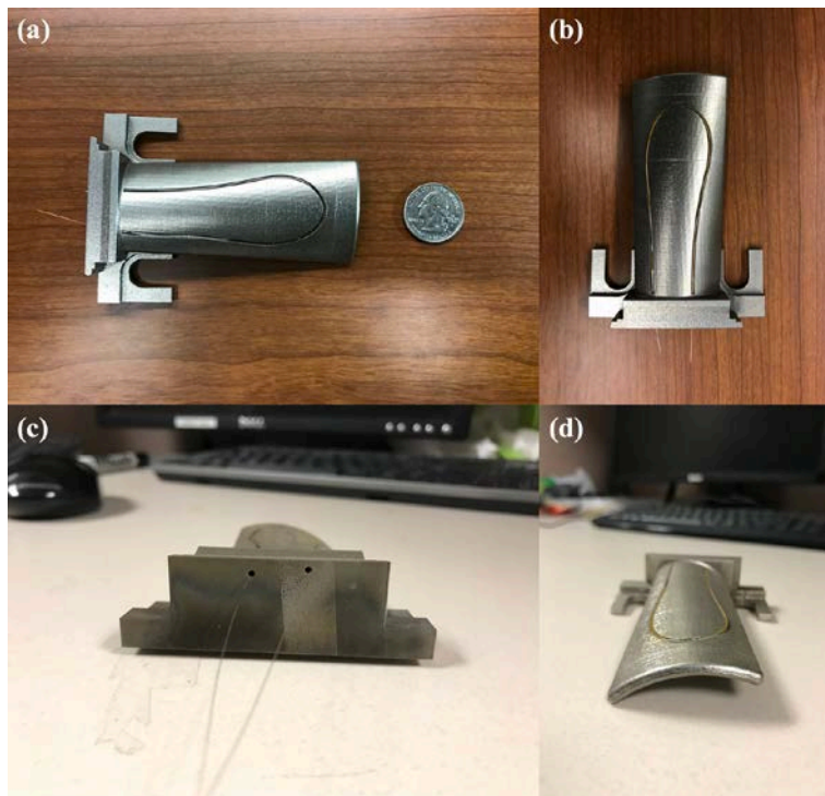
Figure 28 The Ni electroplated optical fiber was transferred into the turbine blade.
