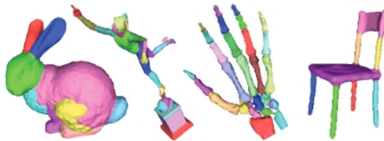
Figure 2.7.: Randomized Cuts for 3D Mesh Analysis [GF08]. Each distinct mesh segment is colored uniquely.
