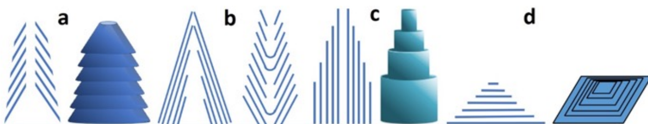
Figure 12: Sketch of the three ways to generate graphenic morphologies whose conical forms are driven by the texture, i.e., the orientation of the graphene layers with respect to the cone axis. (a) and (b) three different textures for graphene sheets oblique to the cone axis; (c) graphene sheets parallel to the cone axis; (d) graphene sheets perpendicular to the cone axis. The line-drawings aside the 3D models sketch the way the inner texture of overall conical morphologies may look like when seen as projected images such as obtained by HRTEM. Although the 3D models in (a) , (c) , (d) hypothesize a stack configuration, the projected textures would look the same in case of a cone-helix configuration.
