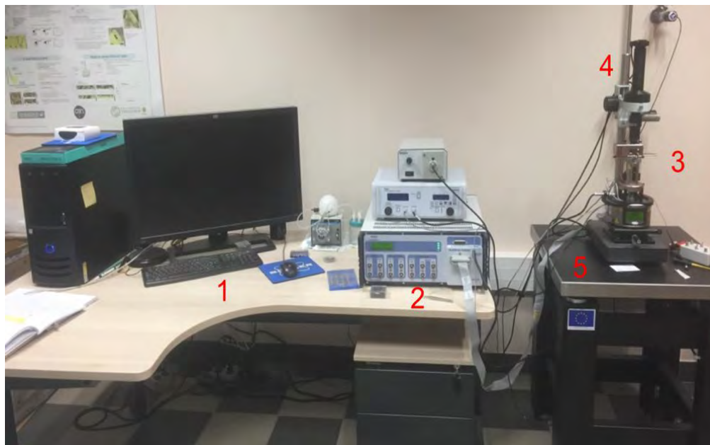
Figure 2-22. Bruker multimode8 complete hardware setup. 1: PC (monitor, CPU, keyboard and mouse), 2: Nanoscope V controller, 3: Multimode V8 Scanning Probe Microscope (SPM), 4: The OMV-UNIV optical viewing system (helps for aligning Multimode SPMs), 5: VT-102-2 which is an air table for vibration isolation to set the SPM on.
