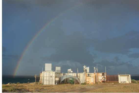
Figure 3.1 – Barbados Cloud Observatory in February 2019. While the Raman lidar and the Ka-band radar are located on the containers to the left, the MWR HATPRO is installed further to the right next to the ceilometer, and the W-band radar is located on top of the middle container. The radiosonde preparing station is located in the center, while soundings are launched from outside of the fenced area.
