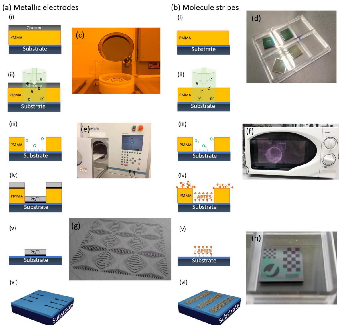
Figure 3-1: Lithography and lift-off technology for sensor creation (a) and patterned molecule deposition (b) consisting of (i) PMMA and (optional) chrome coating, (ii) e-beam writing, (iii) chrome etching, development and oxygen plasma/ozone cleaning, (iv) metal vaporization/molecule deposition, (v) lift-off; (vi) represents the sample with the resulting electrodes/stripes of molecules. Additional pictures of (c) spin coater, (d) 10 x 10 mm 2 SiO 2 and Pt samples, (e) plasma oven, (f) ozone generator, (g) wafer with 9 sensors, and (h) patterned sample for molecule deposition.
