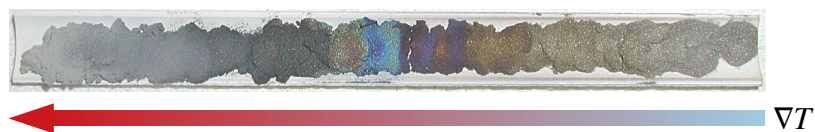
Figure A.2: Boat with titanium powder. Photograph of a boat with (partially) oxidized titanium powder after heating in a tube furnace with argon gas flow. The arrow indicates the temperature gradient in the furnace.
