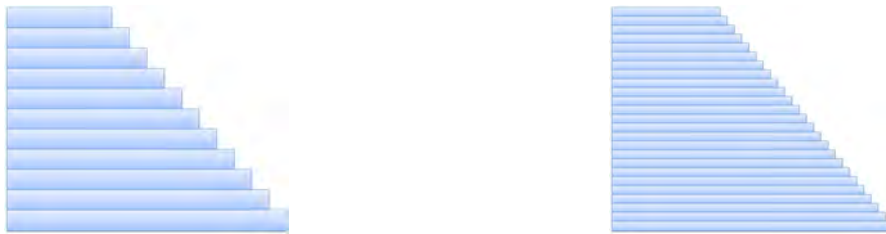
Figure 1.10. Influence of thickness for spread layers on the surface appearance of parts
