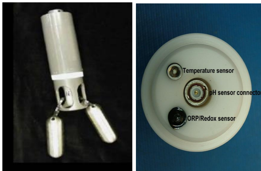
Figure 10. Wireless data logger (Dascor, Escondido, CA, USA) used for in vivo measurements of ruminal E_h and pH (Method 2).
