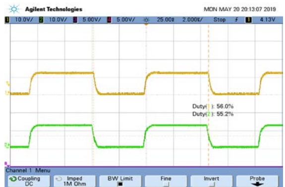
Fig. 17. Experiment I – Sp-Sc connection PWM
