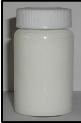
Figure 2.5 Appearances of the BMF samples in glass jars. Polystyrene particles stay suspended in the mixture fluid after 2 weeks (glycerin and water-soluble silicone oil) (Yoshida et al., 2012).
