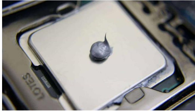
Figure 2.4 Example of thermal paste that has been used in electronic devices (Kohli, Sobczak et al. 2001)
